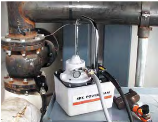
▶ The PA17 used with a flange spreader
