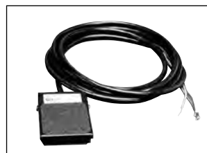
251660 – Foot switch with 10 ft. cord. Single pole, double throw, 15 amp @ 125-250VAC. Wt., 1.0 lb.
