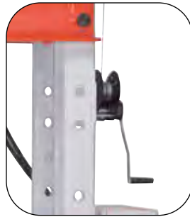
Winch provides easy positioning of press bed
