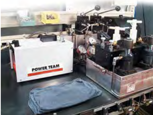
▶ The PA50 used in a work-holding environment
