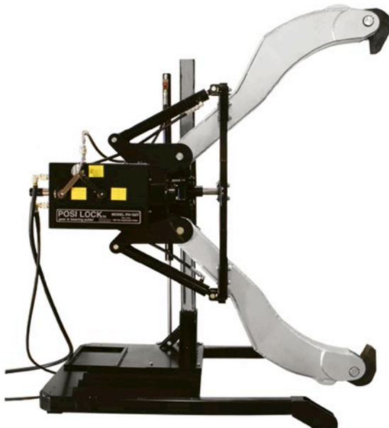
Vertical 91-Ton Hydraulic Puller | PTPH-102TV
