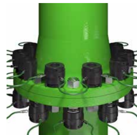
Set up using a 100% tensioning coverage. All the bolts are tensioned at the same time. The particular shape of the interconnecting hoses used to link all the bolt tensioners in the 100% and 50% tool coverage configurations is named "daisy chain"
