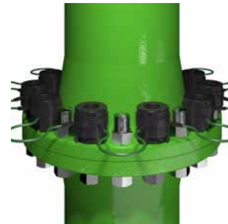
Set up using a 50% tensioning coverage. A half of the bolts are tensioned simultaneously, then the tools are moved to the second half of the bolts.
